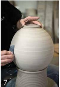
Shave the trimming marks using a metal rib held at close to a right angle against the pot.
