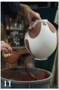
The shape of the pot, glaze viscosity, velocity, and angling of the pot changes the poured shape.
